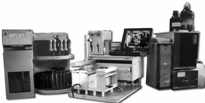
Fig. 1. The hardware setup: coupling of PLE, automated SPE and HPLC (from left to right: ASE 200, ASPEC XLi, HPLC).
